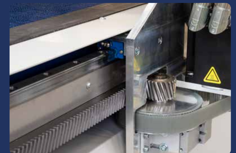
Gear drive for maintenance-free and precise running of the bridge incl. cutting head
