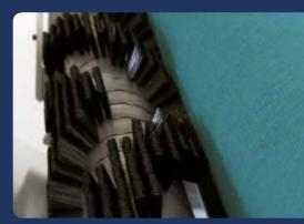
Cleaning brush: The optional cleaning unit eliminates cutting residues.
